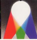
The RSVP doesn't require a three-color dot arrangement to attain true color Instead, red, green and blue beams of light converge and overlay one another, producing continuous tone; rich, saturated hues; and subtle, accurate gradations of gray.
